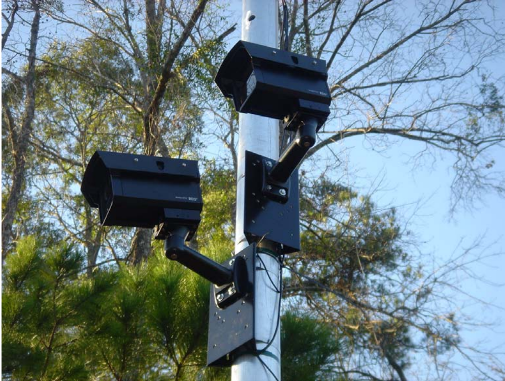
Figure 3.2 – Installed License Plate Reader
